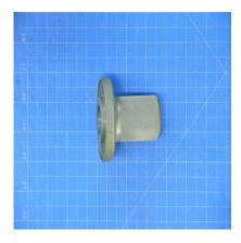
T103263-101 - TAIL ROTOR DRIVE 90 DEGREE GEARBOX BEARING REMOVAL BAR, RENTAL TOOL, FOR USE ON BELL HELICOPTERS
