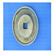
T103071 - MAIN TRANSMISSION LOWER COLLAR GEAR DUPLEX BEARING NUT WRENCH, RENTAL TOOL, FOR USE ON BELL HELICOPTERS
