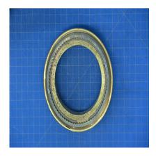
T103037-101 - MAST NUT POWER WRENCH ADAPTER ASSEMBLY, RENTAL TOOL, FOR USE ON BELL HELICOPTERS
