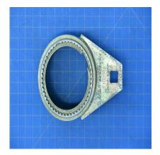
T103011 - TAIL ROTOR SPLINED WRENCH, RENTAL TOOL, FOR USE ON BELL HELICOPTERS
