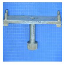
T101883 - MAIN TRANSMISSION FIXTURE SET, RENTAL TOOL, FOR USE ON BELL HELICOPTERS
