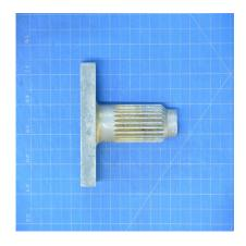
T101568 - SPUR AND SUMP QUILL WRENCH ASSEMBLY, RENTAL TOOL, FOR USE ON BELL HELICOPTERS
