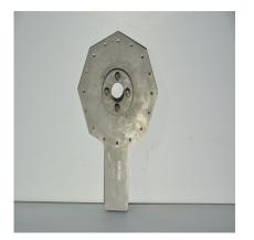
T101563 - 90 DEGREE GEARBOX CASE AND SHAFT HOLDING FIXTURE, RENTAL TOOL, FOR USE ON BELL HELICOPTERS
