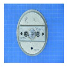
T101420 - DRIVESHAFT COUPLING HOLDING FIXTURE, RENTAL TOOL, FOR USE ON BELL HELICOPTERS
