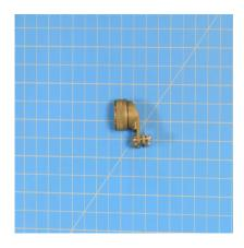
MS3418-12A - Backshell, Circular Connector, 90 Degree
