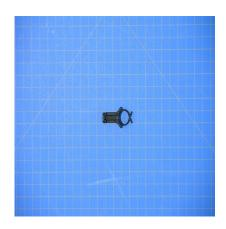
M81969/14-06 - Contact Insertion/Extraction Tool
