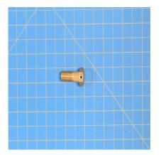
AN6H7A - Bolt, Machine, AN Standard, 5/16" Grip ,61/64" Length, 3/8-24 Thread
