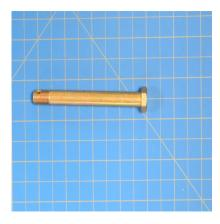
AN6-37 - Bolt, Machine, AN Standard, 3-5/16" Grip , 3-61/64" Length, 3/8-24 Thread
