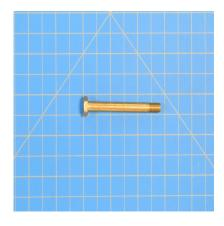
AN4-25A - Bolt, Machine, AN Standard, 2-3/16" Grip , Length 2-21/32", 1/4-28 Thread
