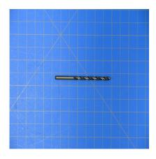
01-021 - Drill Bit, Cobalt, Size 21, 2-1/8" Flute Length, 3-1/8" Total Length, Made to NAS 907 Type J Specifications
